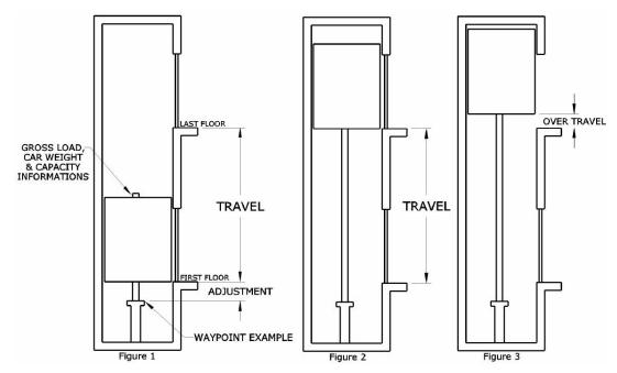
These values are usually written on the inside wall of the elevator or on the top beam over the elevator (see figure 1). The gross load must include the capacity.
